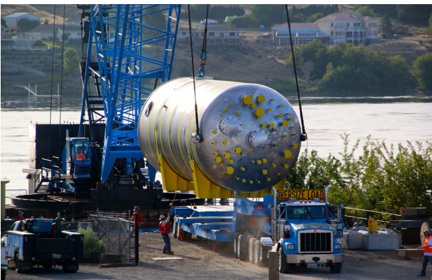
A 35 foot high and 16 foot in diameter stainless steel test vessel arrives at the Port of Benton's High Dock before its delivery to the Atkins Engineering facility.
