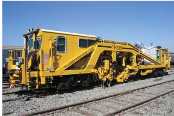
Tamper – Lining & Surfacing Track
